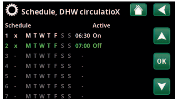
Menu: "Advanced/Settings/DHW Tank/Schedule, DHW circulation". In the example above, "DHW circulation" is activated every week - Monday to Friday between 06:30 and 07:00.
