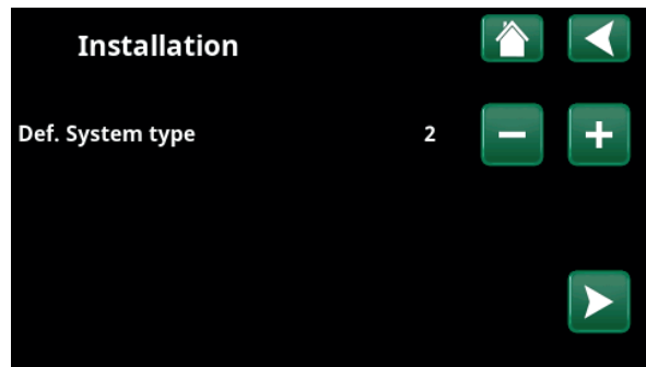
4. Select the system type using the plus/minus (+/-) buttons. Confirm with the "right" directional arrow.
