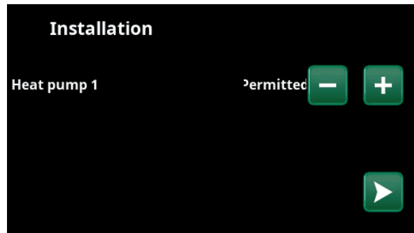
6. Specify whether Heat pump 1 is permitted or blocked. For "Permitted" press plus (+). For "Blocked" press minus (-). Confirm with the "right" directional arrow.
