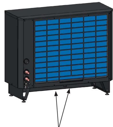
Condensate tray and condensation water drain.
