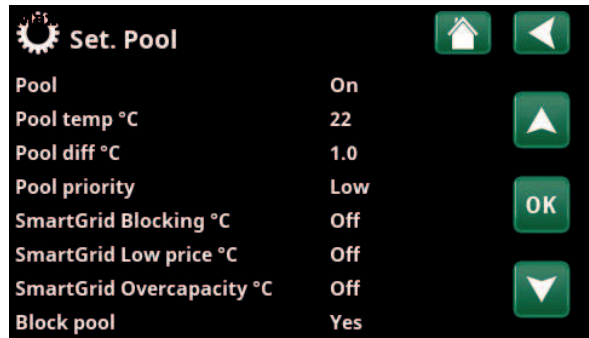
Menu: "Installer/Settings/Pool". Activate this function via an external control signal or a schedule.
