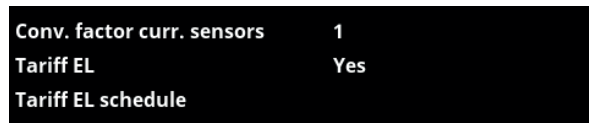
Menu: "Installer/Settings/Additional heat". Setting "Tariff EL" via an external control signal or a schedule.
