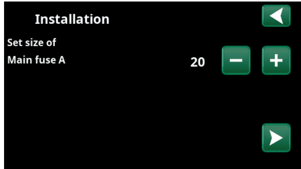
4. Select the size of the main fuse using the "+" and "-" buttons. Confirm with the "right" directional arrow. For more information about settings, refer to the "Advanced/Settings/Immersion heater" chapter.
