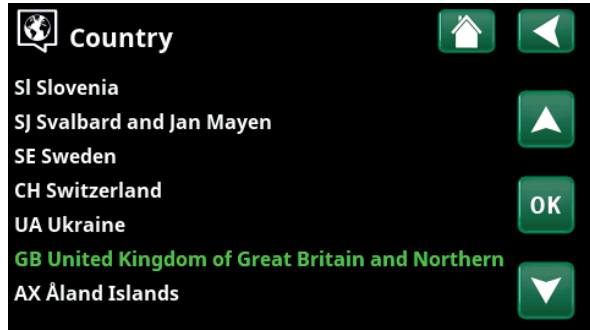
2. Select the country where the heat pump is installed. Press OK to confirm.
