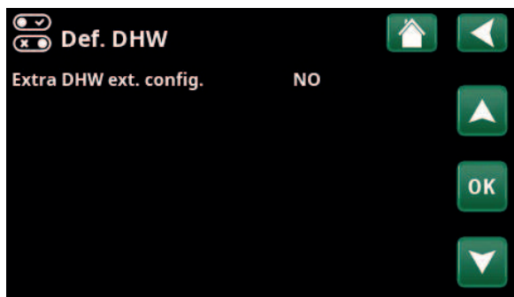
Menu: "Advanced/Define/DHW" On menu bar "Extra DHW", the normal mode is specified for the external control signal ("Normally Open (NO)" or "Normally Closed (NC)").
