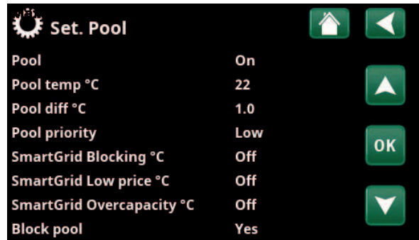
Menu: "Advanced/Settings/Pool". Activate this function via an external control signal or a schedule.
