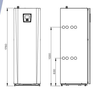
Pipe connection to the right, left, top or rear of the heat pump.
