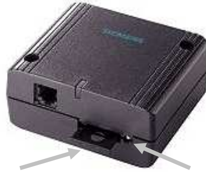
Picture 1. GSM modem with tray and button
